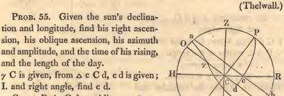
$\therefore$  C  $\gamma = R$  A, C d = oblique asc<sup>n</sup>. and C d measures  $\angle$  C P c,  $..90^{\circ} + CPc = time of rising,$  $2(90^{\circ} + CPc) = \text{length of the day.}$
